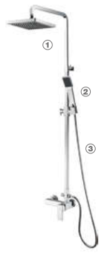
8054 (P38 + S038 + R18 ) ■ ■ Single - lever rain shower mixer (2-function) ① P38 : Shower head , ABS+S/S, 8" ② S038 : Hand shower, ABS, 1-function ③ R18 : Hose, 150cm
