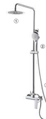
8923 (P72+S019+R18) ■■ Single - lever rain shower mixer (2-function) ① P72 : Shower head, S/S, 8" ② S019 : Hand shower, ABS, 3-function ③ R18 : Hose, 150cm
