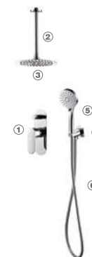
7619-2 (W0219-2+B1009+P72+R27+S019+R18) ■ Concealed - shower mixer (2-function) ① W0219-2: Concealed mixer ② B1009: Shower arm ③ P72: Shower head, S/S, 8" ④ R27: Shower outlet holder, Brass ⑤ S019: Hand shower, ABS, 3-function ⑥ R18: Hose, 150cm
