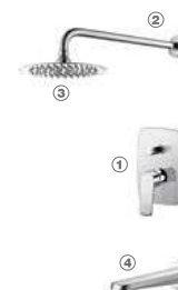
7223-2 (W0223-2+B1011+P72+B2023) ■■ Concealed bath - shower mixer (2-function) ① W0223-2 : Concealed mixer ② B1011 : Shower arm ③ P72 : Shower head, S/S, 8" ④ B2023 : Bathtub spout, Brass, 195mm
