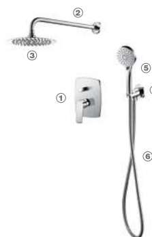
7323-2 (W0223-2+B1011+P72+R27+S019+R18) ■■ Concealed - shower mixer (2-function) ① W0223-2 : Concealed mixer ② B1011 : Shower arm ③ P72 : Shower head, S/S, 8" ④ R27 : Shower outlet holder, Brass ⑤ S019 : Hand shower, ABS, 3-function ⑥ R18 : Hose, 150cm
