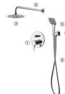
W0514-2+B1011+P72+R27+S050+R18 Concealed - shower mixer (2-function) ① W0514-2: Concealed mixer ② B1011: Shower arm ③ P72: Shower head, S/S, 8" ④ R27: Shower outlet holder, Brass ⑤ S050: Hand shower, ABS, 1-function ⑥ R18: Hose, 150cm
