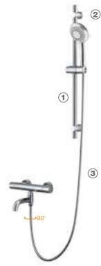
3001 (S08 + S059 + R18 ) ■ ■ Thermostatic shower mixer (2-function) ① S08 : Shower sliding bar, S/S ② S059 : Hand shower, ABS, 3-function ③ R18 : Hose, 150cm
