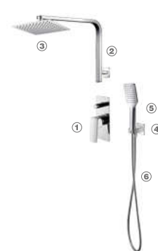
7721-2 (W0221-2+B1295+P73+B2214+S021+R18) ■ Concealed - shower mixer (2-function) ① W0221-2 : Concealed mixer ② B1295 : Shower arm ③ P73 : Shower head, S/S, 8" ④ B2214 : Shower outlet holder, Brass ⑤ S021 : Hand shower, ABS, 1-function ⑥ R18 : Hose, 150cm
