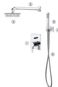
7314-2 (W0214-2+B1113+P70+B2214+S017+R18) Concealed - shower mixer (2-function) ① W0214-2: Concealed mixer ② B1113: Shower arm ③ P70: Shower head, Brass, 8" ④ B2214: Shower outlet holder, Brass ⑤ S017: Hand shower, Brass, 1-function ⑥ R18: Hose, 150cm
