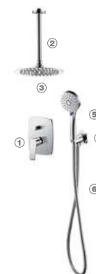
7623-2 (W0223-2+B1009+P72+R27+S019+R18) ■■ Concealed - shower mixer (2-function) ① W0223-2 : Concealed mixer ② B1009 : Shower arm ③ P72 : Shower head, S/S, 8" ④ R27 : Shower outlet holder, Brass ⑤ S019 : Hand shower, ABS, 3-function ⑥ R18 : Hose, 150cm
